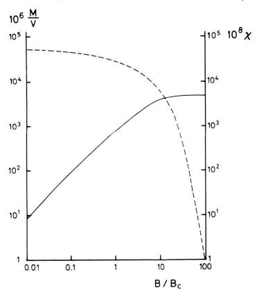
Figure 1 The magnetization per volume  $(M/V \times 10^6)$  on the left axis) and the magnetic susceptibility  $(\chi \times 10^8)$  on the right axis) are plotted as a function of the magnetic field B in the high field range between  $0.01B_c$  and  $100B_c$ . M/V is plotted with the solid curve and  $\chi$  is drawn with broken lines.
