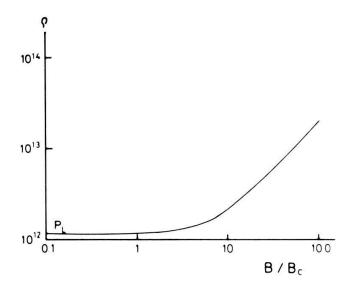
Figure 2 Variation of particle and anti-particle number density as a function of external magnetic field B for the fixed temperature of 511 KeV.
