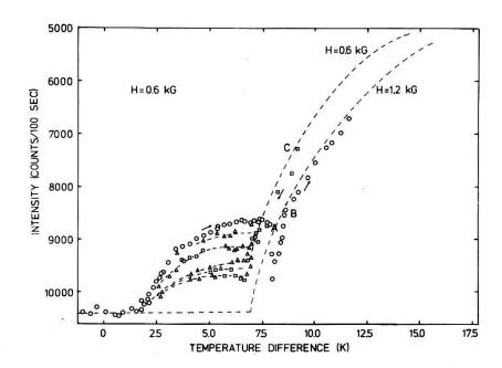
Fig. 3. Neutron intensity versus temperature difference for H = 600 G. Curves drawn for 1.2 kG and 600 G are taken from Fig.1.Triangular symbols give experimental points at levels reached by manipulation of field and gradient.
