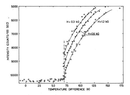
Fig. 1. Neutron intensity versus temperature difference between lower and upper plate, showing threshold to steady flow regime for 1.2 kG. Data points for the two lower fields in oscillatory regime are given in figures below.
