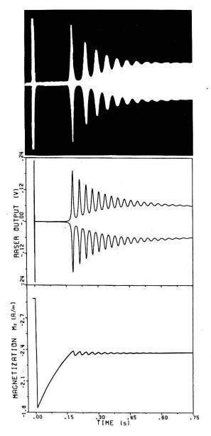
Fig. 1. Raser transients after tuning (Q-switching)
