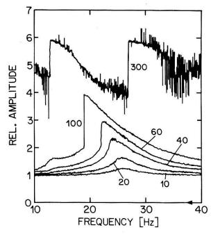
Fig.5. Experimental low-frequency response curve of a modulated raser in function of the drive frequency f for different values of the modulation strength F.
