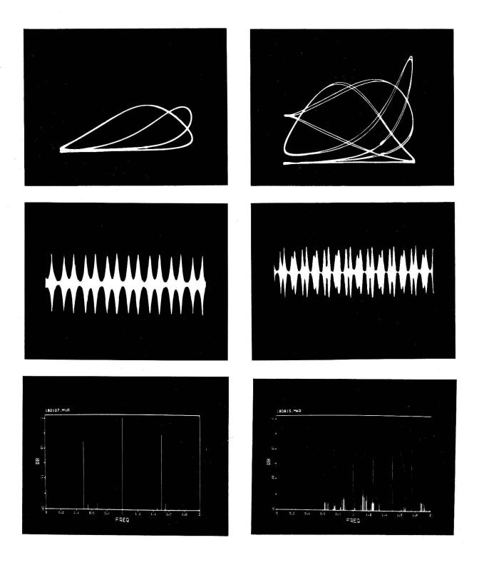
Fig. 3a. Experimental phase-space portraits, time response, and power spectra of a modulated raser in a limit-cycle behavior of period-2 and 4 with erratic noise. The portraits depict the raser output vs. modulator signal.
