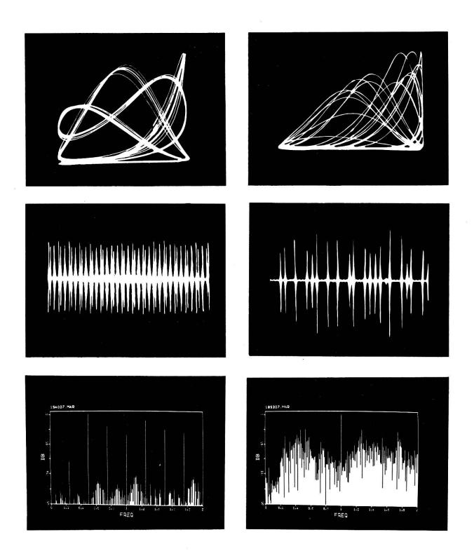
Fig. 3b. Experimental phase-space portraits, time response, and power spectra of a modulated raser in a weakly noisy period-8 limit-cycle and in a chaotic state.
