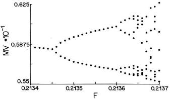
Fig. 7. Bifurcation diagrams for a modulated raser. F refers to the modulation of the DNP pump. The blow-up to the left shows clearly the two pitchfork bifurcations from a period-16 to period-32 and period-32 to a period-64 limit-cycle.
