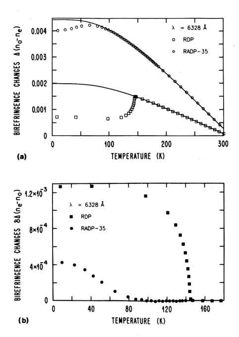
Figure 3. Examples of the birefringence anomaly  $\Delta(n_0-n_e)$  at x=0 and x=0.34. In (a), the solid line is a fit to the high-temperature points that gave Debye temperatures of 424 K for RDP and 415 K for RADP-35, respectively. In (b), the difference between the low-temperature extrapolation of the anharmonic behavior and the measured data is shown.
