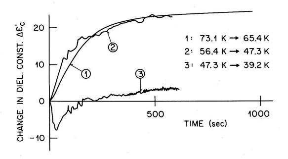
Figure 4. Time development of the polarization current obtained by "step" cooling RADP-35 under a constant static field of 117 V/cm. The cooling has approximately the shape of curve 1. It is slow due to the poor thermal contact (He exchange gas). The starting and final temperatures are given for each step. The vertical axis is in units of effective changes of the "static" dielectric constant. A positive sign means that  $\epsilon_{\rm C}$  increases on cooling.
