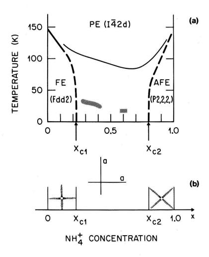
Figure 1. (a) Phase diagram of RADP. Heavy solid line: apparently continuous transition; dashed line: apparently first-order transition on cooling; thin solid line: first appearance of anomalies at  $T_M$ ; shaded region: second appearance of anomalies at  $T_g$ . (b) Near forward scattering patterns of the FE (0  $\le$  x  $\le$  x<sub>c1</sub>) and AFE (x<sub>c2</sub>  $\le$  x  $\le$  1) domains when the  $\alpha$  axes of the BCT unit cell are oriented as shown.
