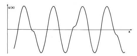
Fig. 1 Normalized atomic displacement  $u(x) = \sin(\phi(x))$  for  $k=\sin^{-1}(89^{\circ})$ .
