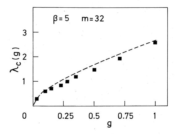
Fig. 3. The critical value  $\lambda_{C}$  of the electron-phonon coupling as a function of the phonon gap g at the Brillouin zone boundary. The dashed line is a theoretical result obtained from comparison of weak and strong coupling expansions.
