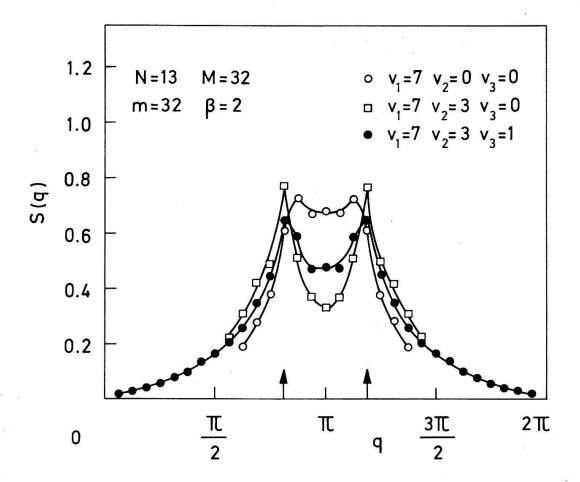
Fig. 1. The wave vector dependent static structure factor S(q) of a one-dimensional system of interacting spinless fermions for several values of the near-neighbor couplings  $V_{\ell}$ . Solid lines are guides to the eye only.
