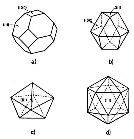
Figure 1 : a) cubooctahedron with (111) hexagonal faces or truncated octahedron, b) cubooctahedron with (111) triangular faces, c) decahedron,
