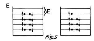
5 - Quantization effect for delocalized electrons in small metallic clusters.
