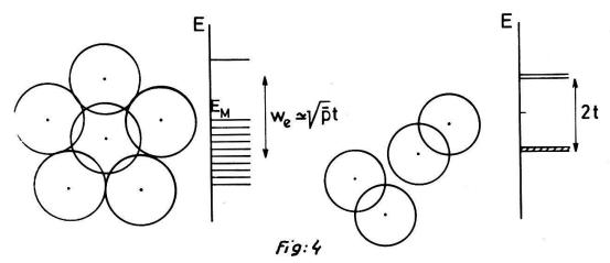
4 - Band structure of close packed structures, compared with the two levels systems of dimers (monovalent metals).
