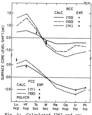
Fig. 4: Calculated [26] and experimental shifts (Table I),  $\Delta_c$ , for different crystal surfaces of the 5d transition metals.
