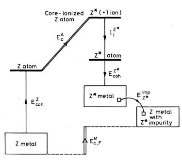
Fig. 1: Diagram showing the connection between the atomic core ionization energy,  $E_c^A$ , and the metallic core level binding energy,  $E_{c,F}^M$ .
