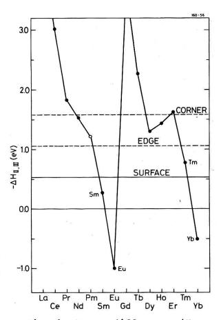
Fig. 6: Energy difference,  $\Delta H_{\Pi,\Pi}$ , between the divalent and trivalent state of the rare-earth metals. For the elements where  $-\Delta H_{\Pi,\Pi}$  falls below the critical line labelled 'surface', the surface will be divalent. Similarly for the case of an edge or a corner.
