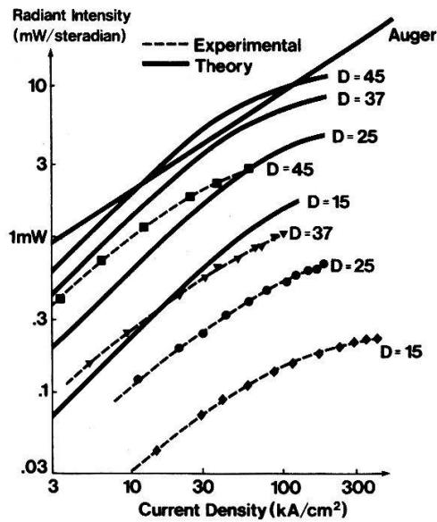
Fig.4: Light vs current showing saturation
