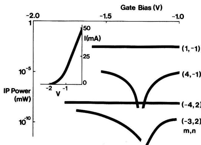
Fig.2: IP power levels and  $I(V)$  (inset)
