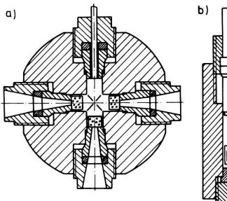
Fig.1. Diamond anvils used for optical [2] or X-ray [3] experiments.
