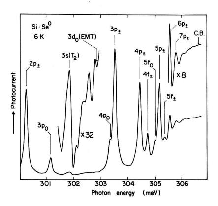
Fig. 5: Enlargement of part of the Si:Se<sup>0</sup> photoconductivity spectrum of figure 4.
