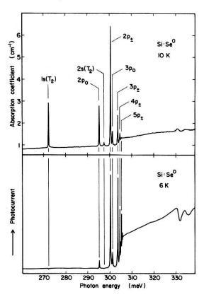
Fig. 3: Fourier absorption and photoconductivity spectrum of selenium doped silicon <sup>16)</sup>.
