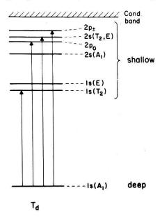
Fig. 2: The lower part of the energy spectrum of a substitutional chalcogenide center in silicon. EMT and symmetry-allowed no-phonon transitions are marked with arrows.
