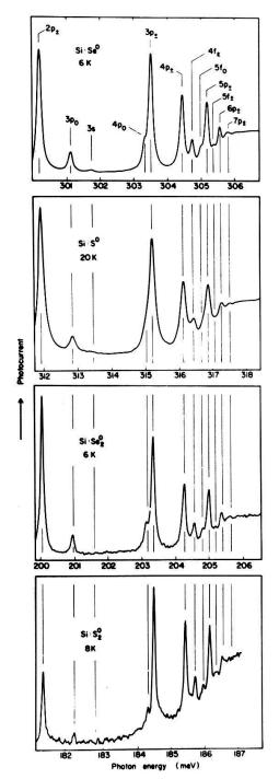
Fig. 4: Photoconductivity spectra of sulfur and selenium doped silicon <sup>16)</sup>, showing transitions from the ground state to the excited states of isolated, neutral impurities on tetrahedral sites (Si:S<sup>0</sup>, Si:Se<sup>0</sup>) and of impurity pairs on trigonal sites (Si:S<sup>0</sup>, Si:Se<sup>0</sup>).
