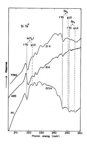
Fig. 10: Comparison of spectra <sup>16)</sup> which have been obtained above the ionization limit in Si:Te<sup>0</sup> using FPAS, Fourier absorption (ABS) and Fourier photoconductivity (PC).
