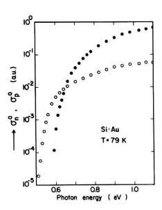
Fig. 1: Optical cross section for electrons and holes versus photon energy for the gold acceptor in silicon <sup>22)</sup> at 79 K.
