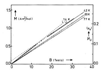
Fig. 5. Magnetization curves of UA12.
