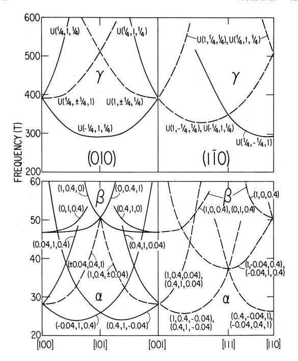
Figure 2. dHvA frequencies associated with the third-zone of the Fermi surface of aluminum (Ref. 15) as a function of field orientation, for magnetic fields in the (010) and (110) planes. The labels on the curves refer to the approximate position of the centers of the relevant orbits in the Brillouin zone as given in Ref. 16. Branches which will separate when the magnetic field does not lie in the (010) or (110) symmetry plane are dashed.
