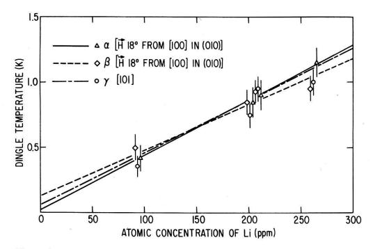
Figure 3. Dingle temperatures (renormalized by electron-phonon interaction) for three third-zone orbits ( $\alpha$  centered at (-0.04, 1, 0.4),  $\beta$  at (0, 1, 0.4) and  $\gamma$  at U(-1/4, 1, 1/4)) as a function of the Li concentration in aluminum. The intercept at zero concentration is due to dislocations and unknown impurities.
