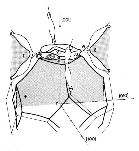
Figure 1. Second-zone hole sheet and third-zone electron monster of the Fermi surface of aluminum. All orbits are drawn for the magnetic field in the [100] direction, except for  $\alpha$  which merges with  $\beta$  for that orientation of the magnetic field and has therefore been drawn for the [110] orientation of the latter.
