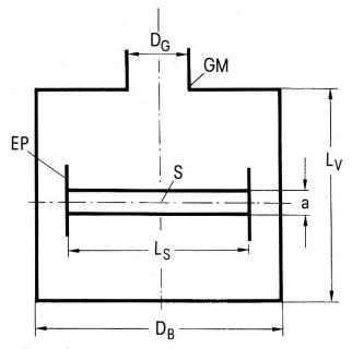
Figure 2 Vacuum-insulated 'conductor-in-box' system (schematically); S specimen NbTi/Cu; EP end plate (on both ends of the NbTi/Cu); GM opening with Gorter-Mellink duct.
