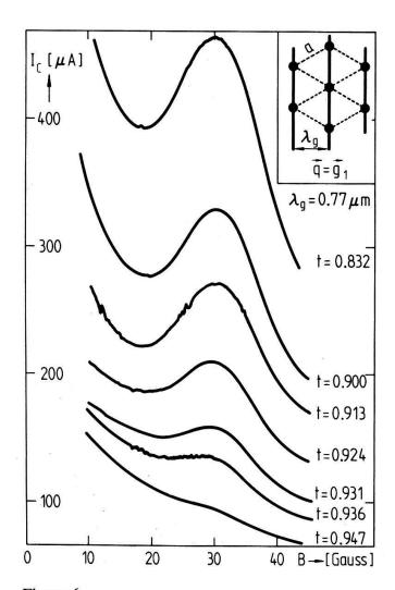
Figure 6 Critical current vs. magnetic field curves of a thickness modulated film (Al2) for different reduced temperatures  $t = T/T_c$ .
