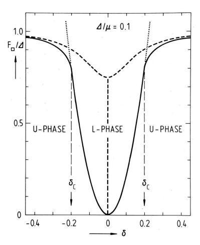
Figure 3 Areal energy density of a 2D lattice in a 1D periodic force field as a function of the mismatch  $\delta$ . The full curve is based on equation (9). The dashed curve follows from a discrete lattice model allowing only for harmonic deformations. In this case the LU-transition occurs at  $\delta = 0$ .
