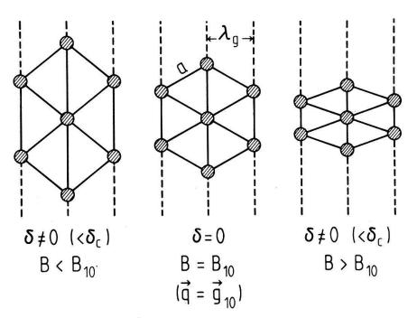
Figure 2 Three different deformation states of the fundamental commensurate  $L_{10}$ -phase.
