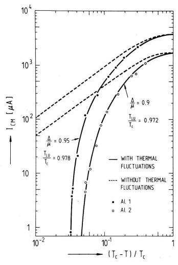
Figure 7 Temperature dependence of the critical currents of thickness modulated films for the fundamental matching configuration  $\vec{q} = \vec{g}_1$ . Theoretical curves are calculated from equation (29) with (full lines) and without (dashed lines) the effect of thermal fluctuations.
