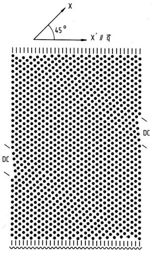
Figure 1 Incommensurate U-phase for  $\delta = 0.13$  ( $B/B_{10} = 0.76$ ). Discommensurations (DC) form a periodic 1D sequence propagating at 45° with respect to  $\vec{q}$ .
