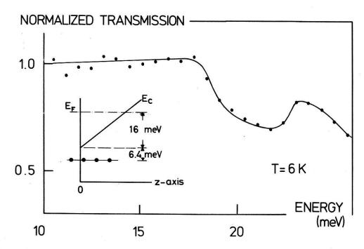
Figure 5 Normalized transmission of sample 430 with respect to bulk GaAs as a function of incident radiation; the insert indicates the schematic energy band at the interface (z = 0).
