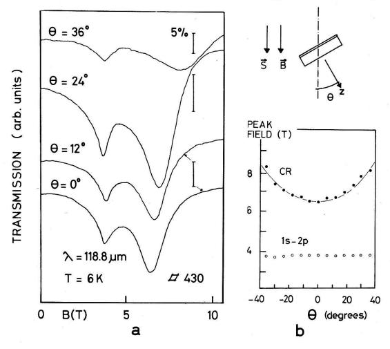
Figure 4 (a) The FIR transmission of sample 430 for various angles. A transmission of 5% is indicated by the vertical bars. (b) The angular dependence of the peak field (CR and 1s-2p) for sample 430. The solid lines represent a  $B/\cos\theta$  dependence.
