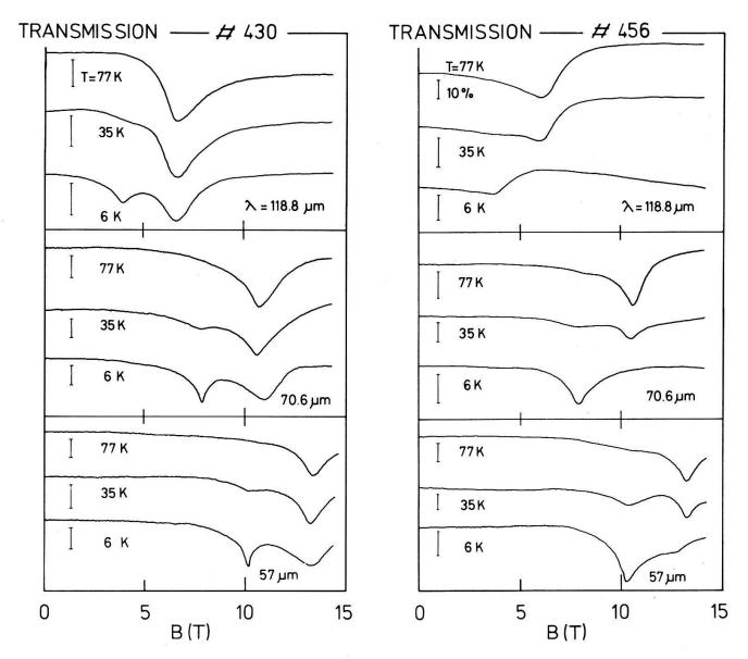
Figure 1 The FIR-transmission of the multilayer n-GaAs-AlGaAs heterojunction sample 430 and the single layer n-GaAs-AlGaAs heterojunction sample 456 for various temperatures and different wavelengths of the incident radiation as a function of the magnetic field. The vertical bars indicate a change in transmission of 10%.
