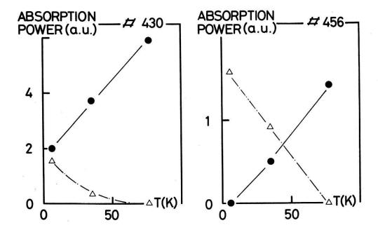
Figure 3 Absorption power as a function of temperature. The triangles  $\triangle$  denote 1s-2p transitions and the full circles  $\bigcirc$  denote the CR transitions. The lines are drawn to guide the eye.
