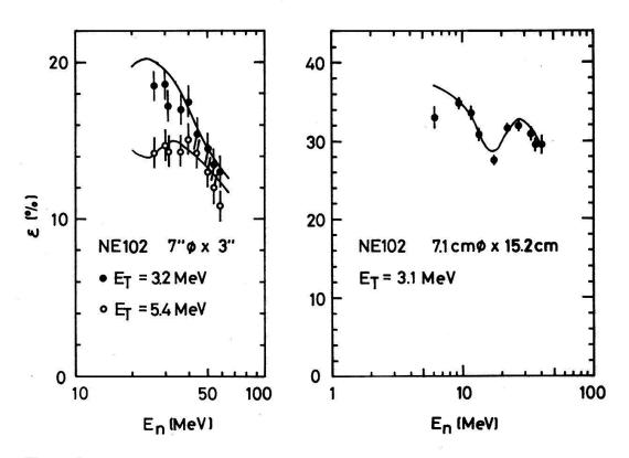
Figure 3 Comparison of the present efficiency calculations (solid lines) with measurements for NE 102 (Ref. [44]:  $7'' \varnothing \times 3''$  and  $E_t = 3.2$  and 5.4 MeV; Ref. [45]:  $7.1 \text{ cm} \varnothing \times 15.2 \text{ cm}$  and  $E_t = 3.1 \text{ MeV}$ ).
