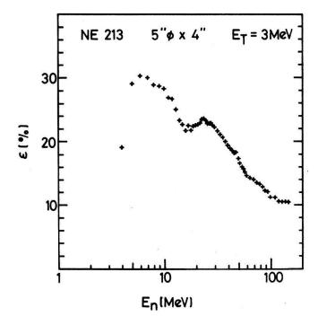
Figure 4 Present neutron detection efficiency  $\varepsilon$  for a 5" diameter and 4" thick neutron detector of type NE 213 for a neutron energy threshold of  $E_t = 3$  MeV (equivalent to an electron energy  $E_e = 973$  keV).
