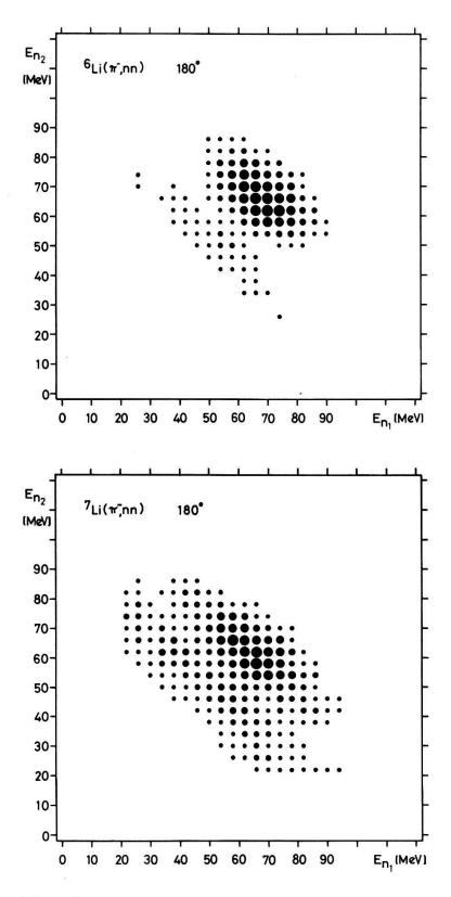
Figure 9 2-dim energy spectra of coincident neutrons ( $E_{n_1}$  and  $E_{n_2} > 20$  MeV) emitted after the absorption of stopped negative pions in  $^6$ Li and  $^7$ Li for an opening angle of 180°. The area of the points is proportional to the intensity  $d^3W/(dE_{n_1}dE_{n_2}d\cos\theta)$ . Both spectra are normalized individually to the maximum of the 2-dim distribution. Points below 10% of the maximum are not plotted.
