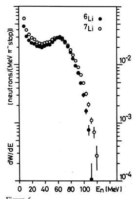
Figure 6 Energy spectra of neutrons ( $E_n > 5 \, \text{MeV}$ ) emitted after the absorption of stopped negative pions in  $^6\text{Li}$  and  $^7\text{Li}$ . The errors shown are statistical only, the error in normalization is 15%. The error in energy is 2.4% at 5 MeV, 3.2% at 10 MeV, 4.4% at 20 MeV, 6.9% at 50 MeV and 10% at 100 MeV.
