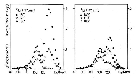
Figure 10 Recoil corrected sum energy spectra of two coincident neutrons ( $E_{n_1}$ ,  $E_{n_2}$ >20 MeV) emitted after the absorption of stopped negative pions in  $^6$ Li and  $^7$ Li for opening angles of 180°, 170° and 160°. Primary p-shell neutrons were defined by the condition  $118 < E_s < 153$  MeV for  $^6$ Li and  $114 < E_s < 146$  MeV for  $^7$ Li. Primary s-shell neutrons were defined by  $82 < E_s < 118$  MeV for  $^6$ Li and  $82 < E_s < 114$  MeV for  $^7$ Li.
