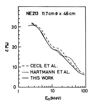
Figure 5 Comparison of the present efficiency calculations with other calculations for NE 213 (Oak Ridge code of Hartmann et al. [21] and the code of Cecil et al. [23, 39]: 11.7 cm  $\emptyset \times 4.6$  cm and  $E_t = 1$  MeV).
