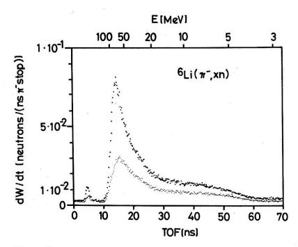
Figure 1 TOF spectrum of neutrons emitted after the absorption of stopped negative pions in  $^6$ Li (large points) and the corresponding background spectrum without target (small points). The spectra are normalized to the number of stopped pions, but are not corrected for neutron detection efficiency. Due to imperfect  $n-\gamma$  discrimination, a small gamma peak can be seen in the measured neutron spectra.
