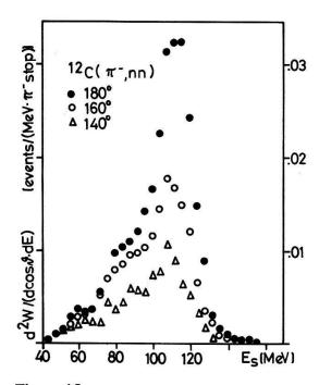
Figure 15 Recoil corrected sum energy spectra of two coincident neutrons ( $E_{n_1}$ ,  $E_{n_2}$ >20 MeV) emitted after the absorption of stopped negative pions in <sup>12</sup>C for opening angles of 180°, 160° and 140°. Primary p-shell neutrons were defined by the condition  $90 < E_s < 128$  MeV.
