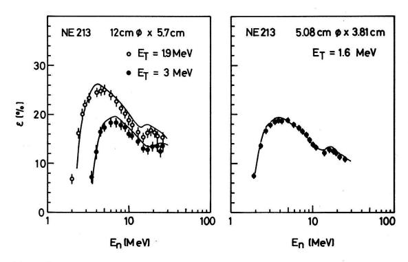
Figure 2 Comparison of the present efficiency calculations (solid lines) with measurements for NE 213 (Ref. [42]:  $12 \text{ cm } \emptyset \times 5.7 \text{ cm}$  and neutron energy threshold  $E_t = 1.9$  and 3 MeV; Ref. [43]:  $5.08 \text{ cm } \emptyset \times 3.81 \text{ cm}$  and  $E_t = 1.6 \text{ MeV}$ ).
