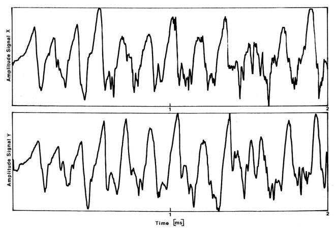
Figure 5 Typical digitized signals from two single probes X and Y operating in the ion saturation current. The probes are positioned to maximum density fluctuation and are azimuthally separated by 60 degrees. The small phase shift of the dominant mode (m = 1) due to the wave propagation between the two probes should be noted.
