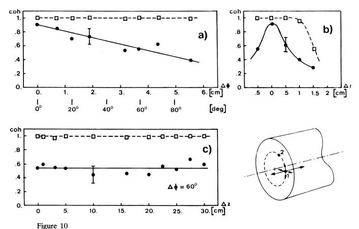
Coherence as a function of the probe separation (sketch) for a turbulent component (11 kHz) (---) and for the coherent wave at 6 kHz (---). One probe is always positioned at maximal fluctuation  $r_{\text{max}} = 3.5$  cm. (a) Azimuthal dependence, (b) radial behaviour, (c) dependence in the z-direction. Here the probes are displaced azimuthally to prevent mutual interference.
