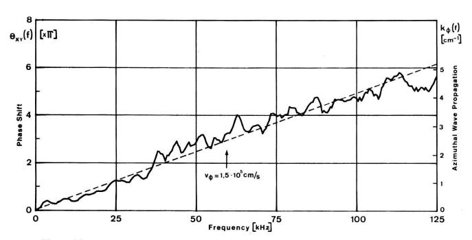
Figure 11 The dispersion relation  $k_{\phi}(\omega)$  determined from the phase spectrum, corresponding to the cross-power spectrum of Fig. 9.  $r_{\text{max}}/R_{\text{pl}} = 0.75$ ,  $\Delta \phi = 60^{\circ}$ .
