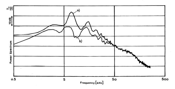
Figure 7 (a) Auto-power spectrum. The probe is positioned at maximal fluctuation  $(r_{\rm max}/R_{\rm pl}=0.75)$ . (b) The random power of the signal. This curve is estimated by subtracting the coherent power from the total power. The Nyquist-frequency is  $f_{\rm Nyq}=250~{\rm kHz}$ .
