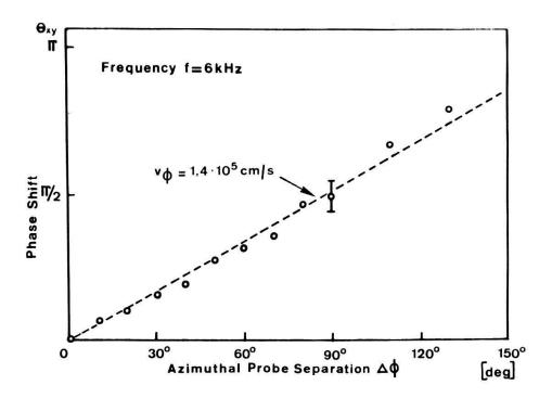
Figure 9 Phase shift between two probes as function of the azimuthal probe separation  $\Delta \phi$ , for the dominant first peak at 6 kHz. The dashed line represents the expected phase dependence for the m=1 mode.
