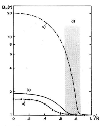
Figure 13 Radial dependence of  $B_N$  at the first magnetoacoustic resonance. (a) Experiment, (b) theory assuming the measured fluctuations, (c) theory excluding turbulence, (d) region of dominant turbulence.
