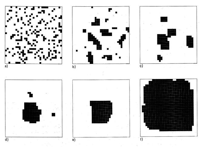
Figure 2 Computer film of nucleation. Torus  $33 \times 33$ ; initial percentage of (-1) spins  $\sim 20\%$ ;  $\alpha = \text{th } (\beta h) = -0.3$ ;  $\gamma = \text{th } (2\beta J) = 0.99$ . Black square indicate (-1) spins.
