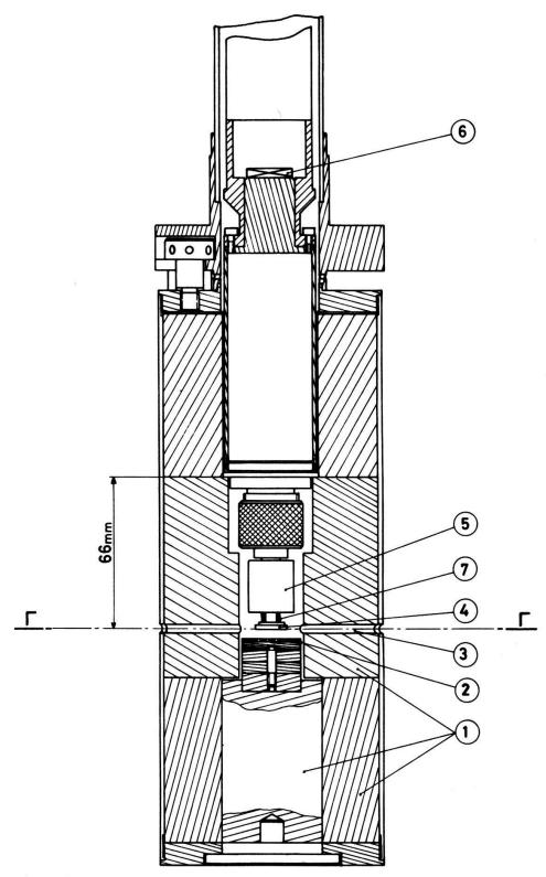
Figure 3. Source-sample assembly. {1}: tungsten shield; {2}: <sup>22</sup>Na source; {3}: hole; {4}: sample; {5}: goniometer head; {6}: mirror; {7}: electric heater.
