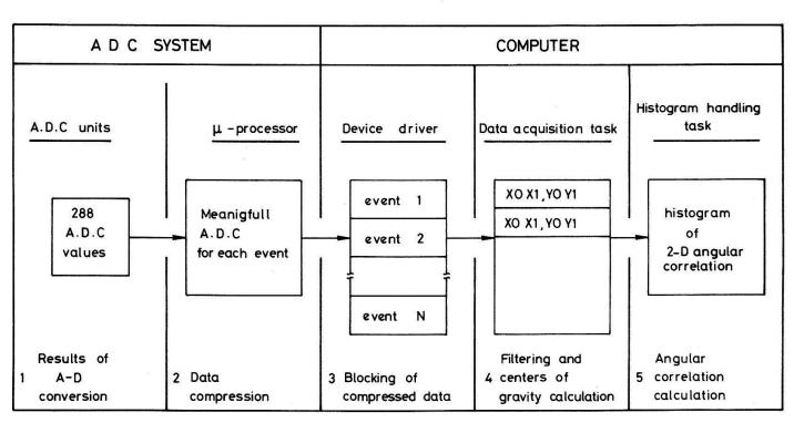
Figure 9. Data flow in the acquisition system.
