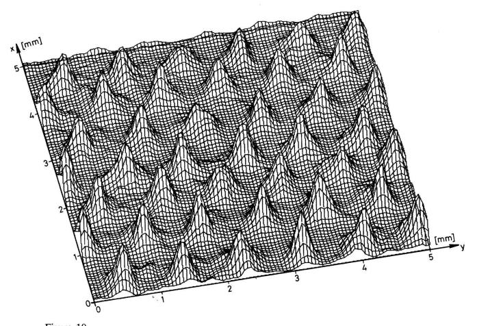
Figure 10. 2-D distribution of calculated position for events striking a  $5 \times 5 \text{ mm}^2$  area of the converter {2} (0.6 mm diameter holes on 0.8 mm pitch). Each peak represents a hole. The hexagonal pattern of holes is clearly visible.
