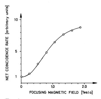
Figure 4. Net coincidence rate vs magnetic field intensity (area of the sample:  $7.5 \times 1.5 \text{ mm}^2$ , source-sample distance: 5.9 mm, distance between detectors: 21 m, T = 4.2 K, source:  $52 \text{ mCi}^{22}\text{Na}$ ).
