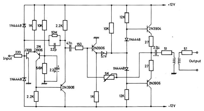
Figure 7. Charge-sensitive amplifier for cathode read-out.
