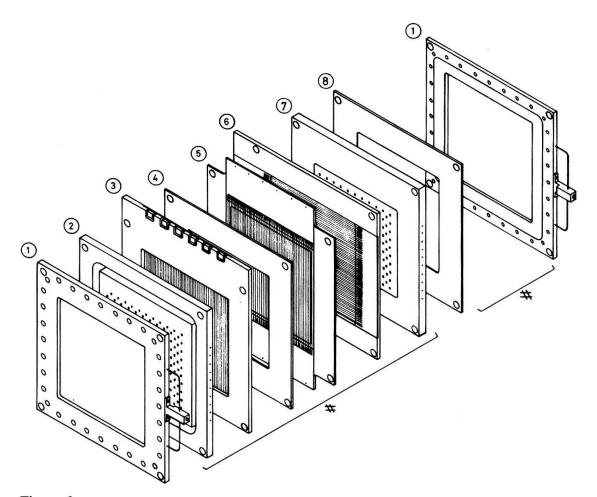
Figure 6. Converters and wire planes layout in a detector; {1}: window frames; {2}, {7}: gamma to electron converters; {3}, {6}: cathode wire-planes; {4}, {8}: spacer frames; {5}: anode wire plane.
