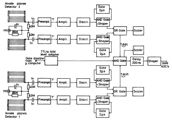
Figure 8. Trigger logic of 2-D ACPAR.
