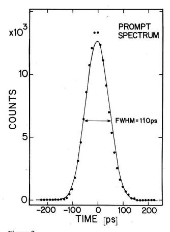
Figure 2 Time resolution spectrum obtained with muons which pass all the detectors without target or degrader. The curve is from a fit to a Gaussian with FWHM = 110 ps.
