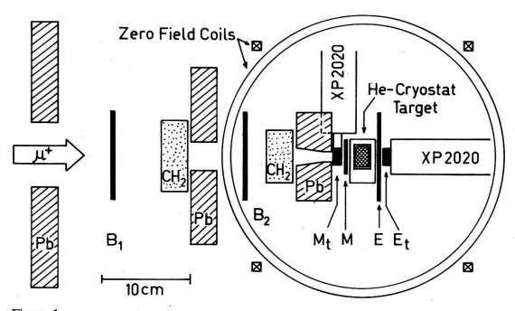
Figure 1 Schematic view of the detector arrangement. Shown are the scintillators (black bars), the lead collimators (Pb), the degrader ( $\mathrm{CH}_2$ ), the cryostat with the target inside and the photomultipliers (XP 2020) of the timing detectors.
