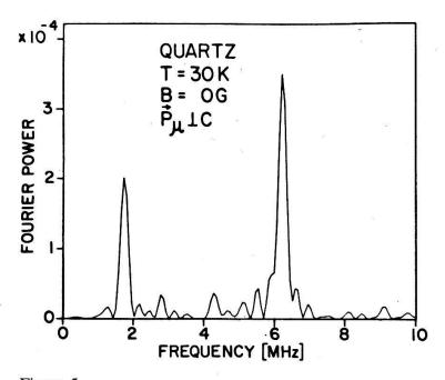
Figure 5 Fourier transform of a spectrum obtained at 30 K with a long time scale, showing the slow transition frequencies.
