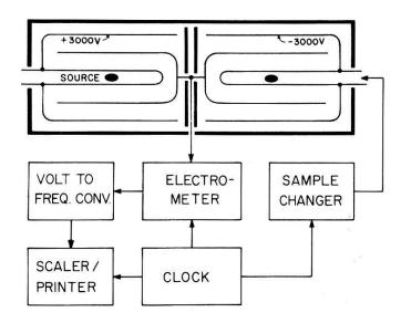
Figure 2 Diagram of the differential ionization chamber.
