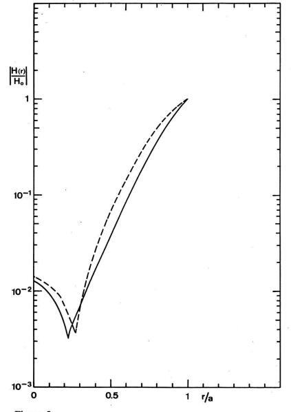
Figure 5 Spatial variation of the magnetic field amplitude in a plasma column under conditions used in ([4], Fig. 5): a = 5 cm,  $\delta_0 = 0.42$  cm, T = 0, 6 eV,  $\nu = 5$ ,  $5 \cdot 10^7$  sec<sup>-1</sup>,  $\omega/2\pi = 7$  MHz. Dotted line is an experimental curve taken from [4] and full line represents the results of calculations with formula (35).
