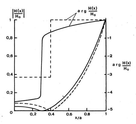
Figure 3 Spatial variation of the amplitude and phase of the magnetic field in the plane case for  $\lambda = 3, 7, \omega/\nu = 5$ ,  $\varepsilon = 15^{\circ}$ . Full lines represent the results of the numerical calculations in [1], dotted lines were calculated from the formula (24).
