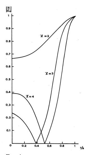
Figure 4 Spatial variation of the amplitude of the magnetic field in the cylindrical case as given by the formula (36) for some values of the parameter  $\kappa = (\pi^{1/6} \lambda^{1/3} a/l)$ , a is the cylinder radius,  $l = u/\sqrt{\omega^2 + \nu^2}$ .
