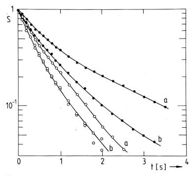
Figure 5 Normalized representation of the variation of the  $F^-$  optical density when F excitation is switched on (O) and off ( $\bullet$ ). (a)  $H_0 = 0$ ; (b)  $H_0 = 0.45$  T.
