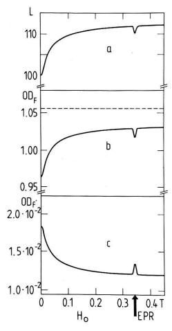
Figure 1 Dependence of the luminescence of the F centers (a), the optical density of the F band (measured at 530 nm) (b), and the optical density of the  $F^-$  band (measured at 629 nm) (c) on the magnetic field H, and under EPR conditions with an optical excitation of the F centers. Dotted line: level of F-optical density without excitation.
