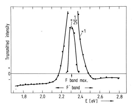
Figure 2 Variation of the transmitted light intensity in several points of the F and F<sup>-</sup> absorption bands, due to a resonant microwave field during F band irradiation.
