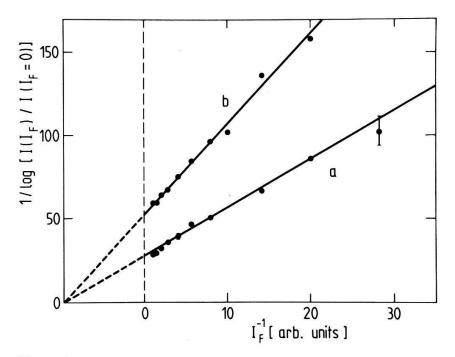
Figure 3 Linearized representation of the transmitted light intensity I in the F band as a function of the excitation light intensity  $I_F$ . (a)  $H_0 = 0$ ; (b)  $H_0 = 0.45$  T.
