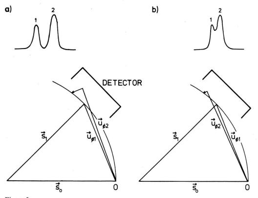
Figure 2 Different resolution in settings for azimuthal angles 0° and 180° for reciprocal vectors  $\mathbf{u}_{\phi 1}$  and  $\mathbf{u}_{\phi 2}$  of unequal lengths.
