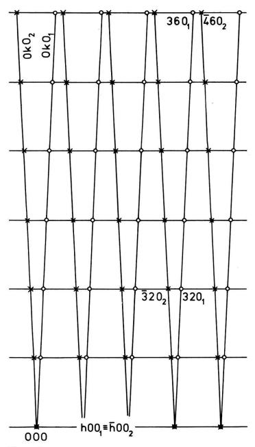
Figure 1 Reciprocal lattices of twinned crystal, hk0 plane. Nearest satellite reflections are  $hk0_1$ ,  $\bar{h}k0_2$  for k < 3 and  $hk0_1$ , -(h+1), k,  $0_2$  for  $k \ge 4$ .
