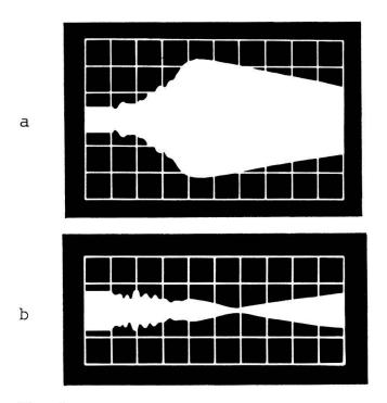
Figur 5 Charakteristische Signale des  $B_z$ -Wellenfeldes; (a) f = 3 MHz, (b) f = 13 MHz; 20  $\mu$ s/E, 100 mV/E.
