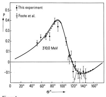
Polarization parameter (P) versus c.m.s. scattering angle ( $\theta^*$ ) at a mean kinetic energy of 310.0 MeV. Full circles: this experiment; quoted errors are statistical. Open circles: results from Reference [7] and [8]. Meaning of the curves as in Figure 3.
