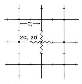
Figure 1 A single random site consisting of a node and s=4 half-bond conductances  $2\sigma$  is embedded in an effective square lattice network whose sites have half-bond conductance  $2\sigma_x$ .
