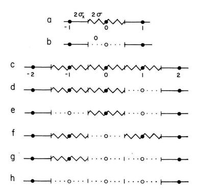
Figure 3 Random bond chains composed of half-bond conductance  $2\sigma$  or 0, imbedded in an effective medium of half-bond conductance  $2\sigma_x$ .
