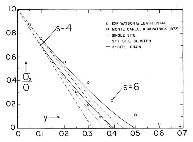
Figure 4 The normalized effective network conductance  $\sigma_x/\sigma$  calculated from various random cluster approximations is compared with experimental data for the site persolation model, for square s=4 and simple cubic s=6 lattices.
