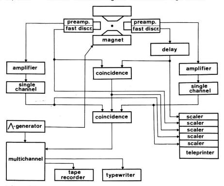
Figure 12 Electronic set-up used for the resonance measurements.
