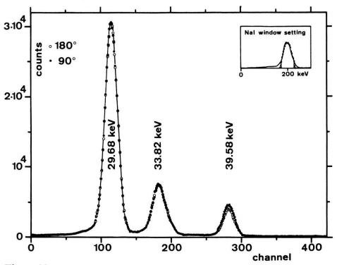
Figure 10 Spectrum of <sup>129 m</sup>Xe, coincident with the 196 keV transition.
