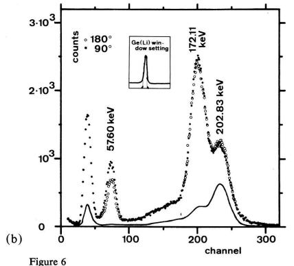
(a) Spectrum of <sup>127</sup>Xe, coincident with the 172 keV transition. (b) Spectrum of <sup>127</sup>Xe, coincident with the 145 keV transition.
