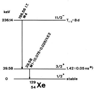
Figure 9 Decay scheme of <sup>129m</sup>Xe, based on Ref. [14].
