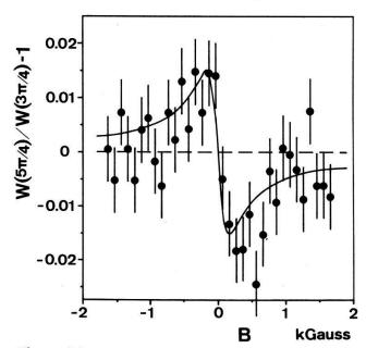
Figure 16  $W(5\pi/4)/W(3\pi/4) - 1$  as a function of the magnetic field for the 172–203 keV cascade in <sup>127</sup>I.
