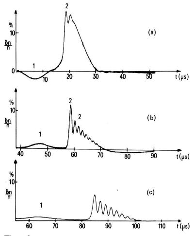
Figure 3 The electron density perturbation  $\delta n/n$  versus time for different distances from the wave excitation point, in the case of the Argon plasma. (a) 34.3 mm, 1 pick up, 2 first soliton; (b) 103.8 mm, 1 reflected ions, 2 solitons; (c) 154.9 mm, 1 reflected ions, 2 solitons.
