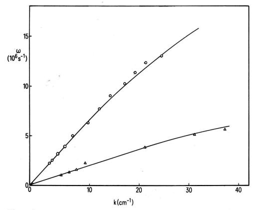
Figure 2 Dispersion relation of small-amplitude ion acoustic wave. (—— Theoretical,  $\triangle$ ,  $\bigcirc$  Experimental values for Argon and Helium, respectively.
