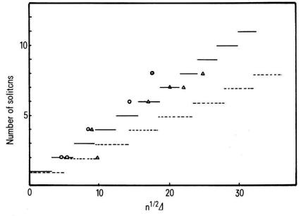
Figure 9 Number of solitons as a function  $\Delta n^{1/2}$ . n is the initial perturbation normalized to the unperturbed plasma density and  $\Delta$  is the width of the pulse in unit of  $\omega_{pi}^{-1}$ . (—— hot ion  $(\theta = 9)$  theory; .... cold ion theory.)  $\bigcirc$ ,  $\triangle$  are the experimental values for Ar and He, respectively.
