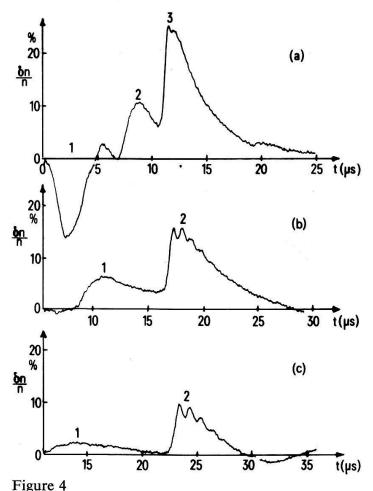
The electron density perturbation  $\delta n/n$  versus time for different distances from the wave excitation point, in the case of the Helium plasma. (a) 53.2 mm, 1 pick up, 2 reflected ions, 3 solitons; (b) 85 mm, 1 reflected ion, 2 solitons; (c) 113.6 mm, 1 reflected ion, 2 solitons.
