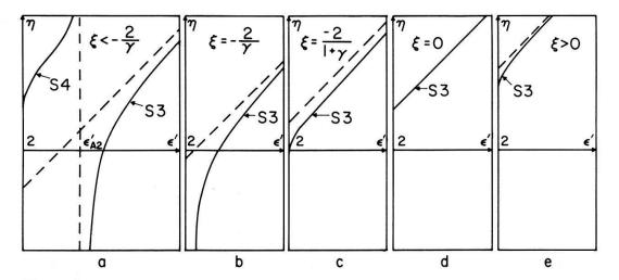
Figure 2 Schematic diagrams of  $\eta$  as a function of  $\epsilon'$  for the two symmetric single spin deviation eigenenergies S3 and S4 above the spin wave band. The  $\epsilon'$  axes begin at 2. The dashed line asymptote in the figures is given by  $\eta = \epsilon' + \xi$ . At the point  $\epsilon' = 2$ ,  $\eta = 2[1 + \xi/(2 + \gamma \xi)]$ . The figures a,
