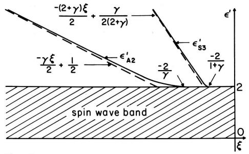
Figure 3 Schematic diagram of the symmetric and antisymmetric single spin deviation eigenenergies  $\epsilon'_{S3}$  and  $\epsilon'_{A2}$  above the spin wave band as a function of  $\xi$ , for the case  $\eta = 0$ . Dashed lines are asymptotes. Slopes are zero of the S3 and A2 curves at  $\xi = -2/(1 + \gamma)$  and  $\xi = -2/\gamma$ , respectively. The parameters  $\xi$ ,  $\gamma$  and  $\epsilon'$  are defined in equation (2.13).
