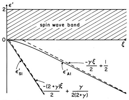
Figure 1 Schematic diagram of the symmetric and antisymmetric single spin deviation eigenenergies  $\epsilon'_{S1}$  and  $\epsilon'_{A1}$  below the spin wave band as a function of  $\xi$ , for the case  $\eta = 0$ . Dashed lines are asymptotes. Slopes of the S1 and A1 curves at  $\xi = 0$  are -1 and 0, respectively. The parameters  $\xi$ ,  $\gamma$  and  $\epsilon'$  are defined in equation (2.13) in terms of the parameters of the Hamiltonian, equation (2.1).
