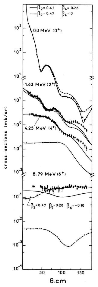
Figure 8 Coupled-channels (rotational model) calculations for the states belonging to the  $K=0^+$  ground state band, namely, the  $0^+$  (g.s.), the  $2^+$  (1.631 MeV), the  $4^+$  (4.25 MeV) and the  $6^+$  (8.79 MeV) with and without a hexadecapole deformation ( $\beta_4=+0.28$ ). The prediction for the  $6^+$  state is slightly improved when a  $\beta_6$  equal to -0.10 is included in the calculations. The optical model parameters (C.C. parameters) of Table II were used.
