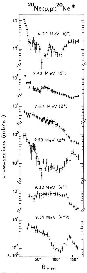
Figure 4 Experimental cross-sections for some positive parity states in  $^{20}$ Ne.
