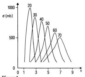
Figure 1 Cross sections for  $^{163}$ Dy(p, xn) interpolated from the tables in *Landolt-Börnstein* [13] and connected with eye-guiding lines. The parameter on the curves is the incident proton energy in MeV. A similar figure obtains from the experimental values [8] for  $^{181}$ Ta(p, xn).
