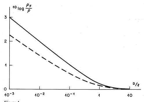
Figure 4 Size effect of thin-film resistivity: Comparison between present theory (full line) and Reuter-Sondheimer theory (broken line).  $\rho_F$  = film resistivity,  $\rho$  = bulk resistivity, D = film thickness, l/2 = electronwave attenuation length (l = mean free path).
