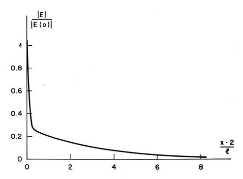
Figure 9 Electric-field amplitude |E| as a function of distance x from the surface of a half-space. |E(0)| = 1; l/2 = electron-wave attenuation length.
