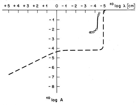
Figure 7 Absorption coefficient A of copper as a function of frequency (expressed in corresponding light vacuum wavelengths,  $\lambda$ ). Experimental (circles between full line) after Biondi [11], theoretical (broken line) according to  $\sigma = \sigma_0 \cdot (1 + j\omega \tau)$  with data  $\sigma_0 = 4.1 \cdot 10^9 \ \Omega^{-1} \cdot m^{-1}$  and  $\tau = 2.4 \cdot 10^{-12}$  sec after Biondi [11].
