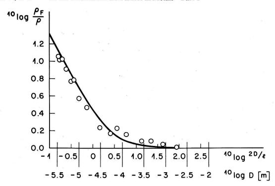
Figure 3 Size effect of thin-film resistivity: Data by Andrew [6] (circles) fitted to theoretical curve (full line).  $\rho_F = \text{film}$  resistivity,  $\rho = \text{bulk}$  resistivity, D = film thickness, l/2 = electron-wave attenuation length.
