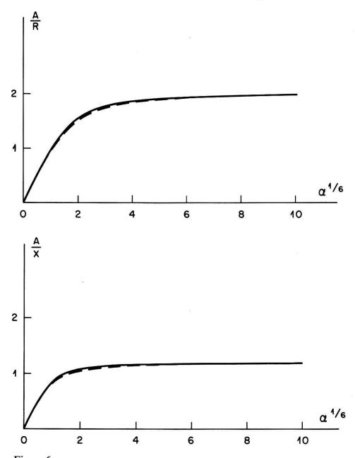
Figure 6 Theoretical dependence of surface impedance R + jX on temperature: Comparison of plots A/R (Fig. 6(a)) and A/X (Fig. 6(b)) against  $\alpha^{1/6}$  according to present theory (full line) and Reuter-Sondheimer theory (broken line). See text for definition of A and  $\alpha$ .
