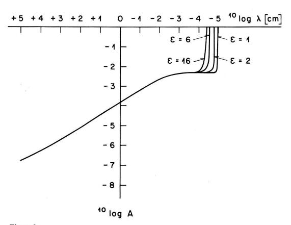
Figure 8 Absorption coefficient A of copper as a function of frequency (expressed in corresponding light wavelengths,  $\lambda$ ), with  $v_F$  (Fig. 8(a)) or  $\varepsilon$  (Fig. 8(b)) as a parameter, according to present theory with data  $\rho l = 6.49 \cdot 10^{-16} \ \Omega \cdot \text{m}^2$ ,  $\sigma_0 = 4.1 \cdot 10^9 \ \Omega^{-1} \cdot \text{m}^{-1}$ .
