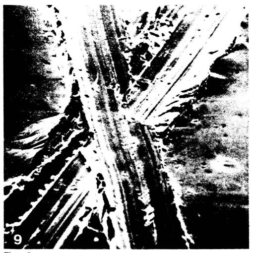
Figure 7 Stereoscan views of freshly abraded nickel surfaces. No. 9: with a diamond tool, magnification: 600; slant angle:  $60^{\circ}$ ; No. 2: with an alumina tool, magnification: 2250; slant angle:  $60^{\circ}$ .
