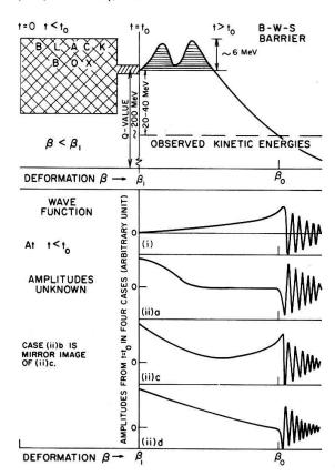
The upper half of the figure represents schematically the observed pre-neutron emission kinetic energies in relation to the potential energy relevant at the tunnelling stage in each of the three models. B-W, B-W-S and QMF refer, respectively to Bohr-Wheeler, Bohr-Wheeler-Strutinski and barrier of Ref. [9] through [12]. The lower half of the figure plots schematically the relevant wave functions corresponding to the potential barrier drawn above it.
