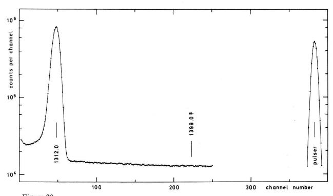
Figure 20 Partial gamma ray spectrum of <sup>160</sup>Dy showing the region around the possible E3 groundstate transition from the second 3<sup>-</sup> level at 1399.0 keV. Energies are in keV.
