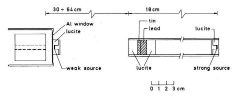
Figure 13 Source to detector geometry for the measurement of the E3 transition and the sum spectrum.
