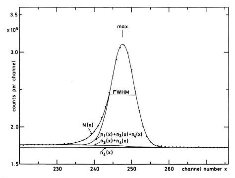
Figure 25 Least squares fit to a typical full-energy peak (432.5 keV transition in the <sup>140</sup>La  $\rightarrow$  <sup>140</sup>Ce decay). The functions N(x) and  $n_i(x)$  are defined in the appendix.
