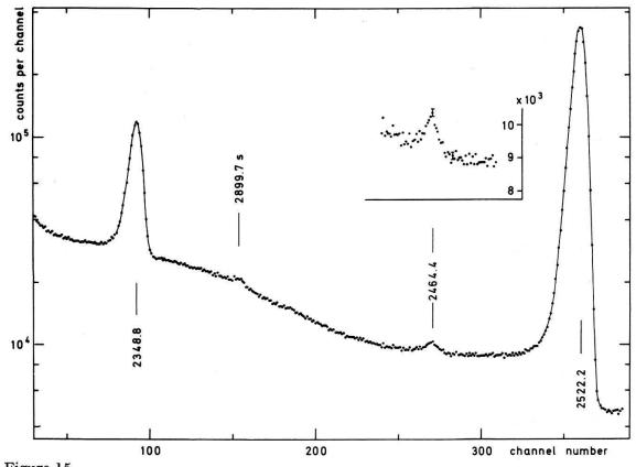
Figure 15 Partial gamma ray spectrum of <sup>140</sup>Ce showing the  $3^- \rightarrow 0^+$  transition. Energies are in keV. s: single-escape peak.
