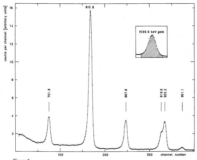
Gamma ray spectrum of <sup>140</sup>Ce in the energy region 700–970 keV measured in coincidence with the 1596.6 keV transition under the angle of 90°. Energies are in keV.
