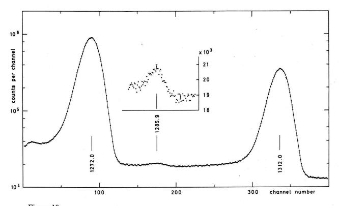
Figure 19 Partial gamma ray spectrum of  $^{160}$ Dy showing the region around the possible E3 groundstate transition from the first 3<sup>-</sup> level at 1286.7 keV. Energies are in keV.
