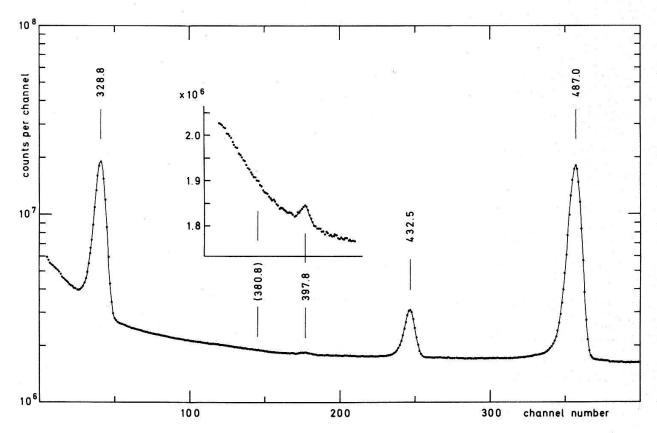
Figure 16 Partial gamma ray spectrum of <sup>140</sup>Ce showing the region around the possible  $3^- \rightarrow 4^+$  transition of 380.8 keV. Energies are in keV.
