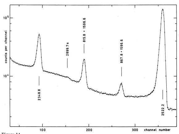
Figure 14 Partial gamma ray spectrum of <sup>140</sup>Ce showing the sum peak of the  $3^- \rightarrow 2^+ \rightarrow 0^+$  cascade. Energies are in keV. s: single-escape peak.
