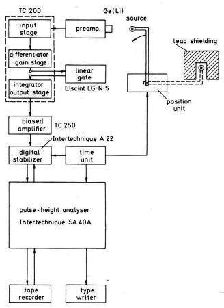
Figure 12 Block diagram of the electronics used for the gamma ray spectroscopy of the decays  $^{140}$ La  $\rightarrow$   $^{140}$ Ce and  $^{160}$ Tb  $\rightarrow$   $^{160}$ Dy. The linear gate has been used only in the search for the  $3^- \rightarrow 4^+$  transition in  $^{140}$ Ce.
