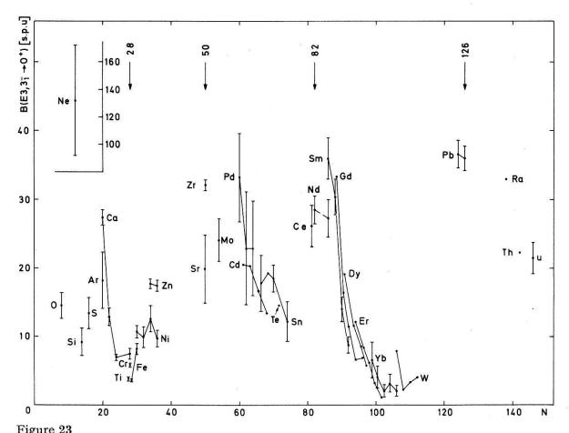
Reduced excitation probabilities B(E3) in single particle units of the lowest  $3^-$  states as a function of neutron number. Isotopes of the same element are connected by solid lines.
