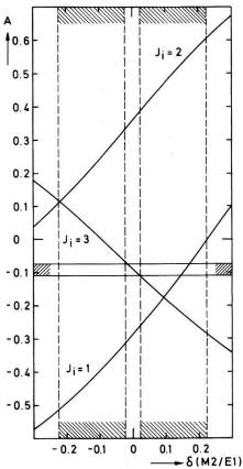
Figure 6 Anisotropy A of the 867.8 keV transition in coincidence with the 1596.6 keV gamma ray as a function of mixing ratio  $\delta$ .  $J_l$  is the spin of the initial level. The hatched regions denote the mixing ratio compatible with the K-conversion coefficient quoted by Baer et al. [22] and the anisotropy from the present work, respectively.
