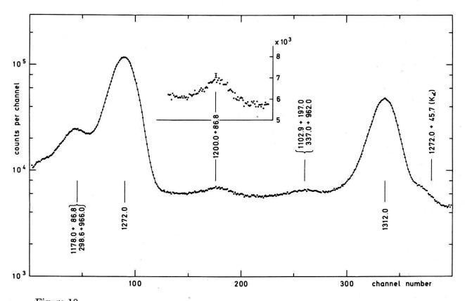
Figure 18 Partial gamma ray spectrum of  $^{160}$ Dy showing the sum peak of the  $3^- \rightarrow 2^+ \rightarrow 0^+$  cascade originating from the first  $3^-$  level at 1286.7 keV. Energies are in keV.
