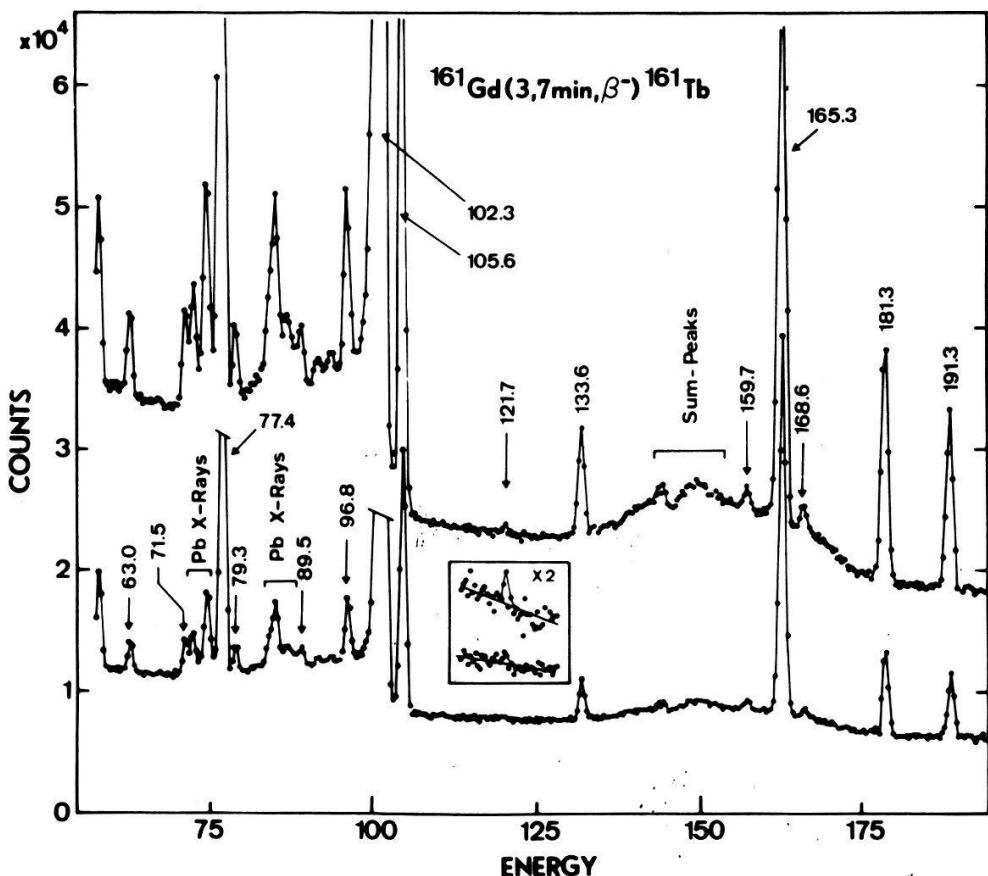
Figure 1 Low-energy part of the  $^{161}\text{Gd}$  gamma-ray spectrum.
