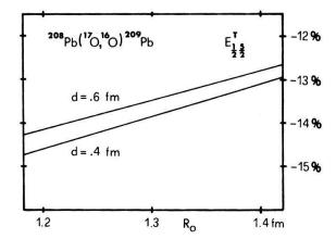
Figure 7 The excitation effect function  $E_{1/2\,5/2}^T$  ( $\vartheta=180^\circ$ ) as a function of the Woods-Saxon parameters  $R_0$  and d.
