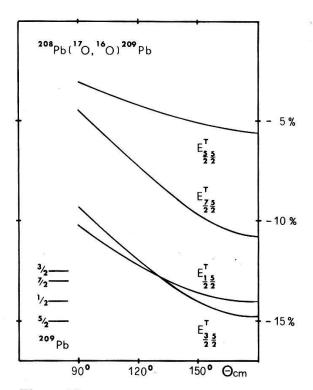
Figure 10 For the reaction  $^{208}$ Pb( $^{17}$ O,  $^{16}$ O) $^{209}$ Pb at a laboratory energy of 70 MeV the effect functions  $E_{zf}^{T}(\vartheta)$  are plotted for the final state  $5/2^+$  at 1.56 MeV in  $^{209}$ Pb. Apart from the reorientation in the  $5/2^+$  state, three higher-lying levels contribute to the excitation effect.
