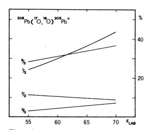
The energy dependence of the target excitation effects in four levels of  $^{209}$ Pb. A value of -.8 barn is used for all non-vanishing E2-couplings.
