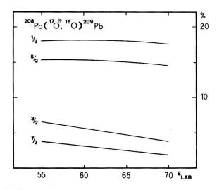
Figure 9 The energy dependence of the projectile excitation effects in four levels of  $^{209}$ Pb. A value of -.07 barn is used for the E2-couplings  $M_{5/2.5/2}^{P}$  and  $M_{5/2.1/2}^{P}$  of  $^{17}$ O.
