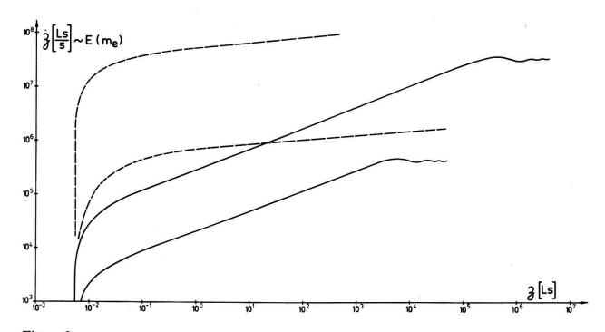
Figure 2  $dz/d\tau = E(m_e) - 1$  as a function of the distance z in units of light seconds. The dotted curves represent the approximate solution of Gunn and Ostriker [1].
