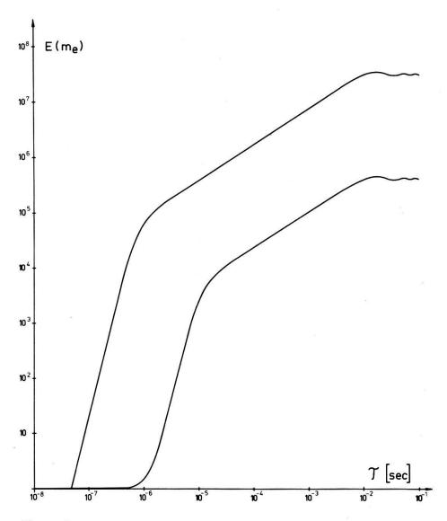
Figure 1 Energy  $E(m_e)$  of the accelerated electrons in units of the electron mass as a function of eigentime  $\tau$ . The upper (lower) curve corresponds to a surface field of  $10^{12}$  (1.5 ×  $10^9$ ) Gauss and a rotation frequency  $\omega \simeq 1.9 \times 10^2 \ {\rm sec}^{-1}$ .
