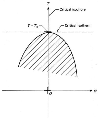
Figure 1 The spontaneous magnetization phase boundary. The two-phase region is shaded.
