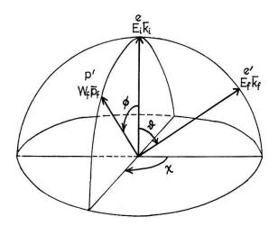
Figure 2 Relation of the momentum of an emitted proton  $p_f$  to the initial and final momenta of the electron  $k_i$  and  $k_f$ .
