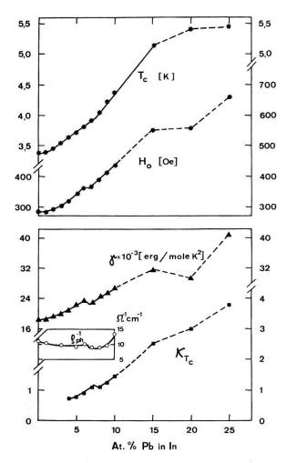
Figure 6 Parameters deduced from magnetization measurements and directly measured values of  $\varrho_{ph}$ .
