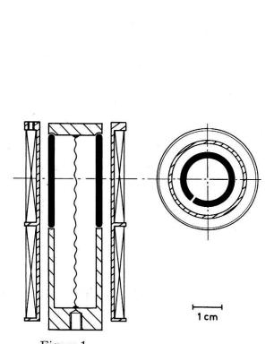
Figure 1 Cylindric sample and pick-up coils as they were put in the measuring capacitance. The actual specimen is the black hollow slit cylinder.
