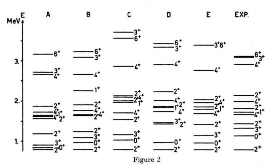
For various values of a and b theory and experiment are compared for states with positive parity in Pb<sup>206</sup>. The range parameter is chosen to be  $\alpha=2$ .. The parameters  $V_0$ , a and b are as follows: Calculation A)  $V_0=.321$  MeV, a=.13, b=.0; B)  $V_0=.212$  MeV, a=.0, b=.775; C)  $V_0=.446$  MeV, a=.13, b=.775; D)  $V_0=.183$  MeV, a=.0, b=.0; E)  $V_0=.355$  MeV, a=.10, b=.776. The introduction of a spin-spin and a tensor interaction yields an appreciable improvement.
