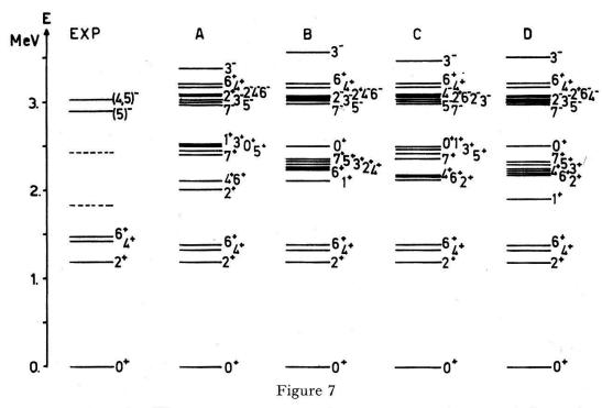
The energy spectrum of Po<sup>210</sup>. A comparison is made between experiment and theory for various values of the parameters a and b. The range parameter is chosen to be  $\alpha=2$ .. Most states are not sensitive to a variation of the parameters a and b. The parameters  $V_0$ , a and b are as follows: Calculation A)  $V_0=.184$  MeV, a=.10, b=.776; B)  $V_0=.128$  MeV, a=b=.0; C)  $V_0=.128$  MeV, a=0, b=.775; D)  $V_0=.211$  MeV, a=.13, b=.0.
