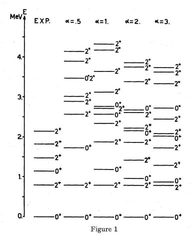
The variation for the states with spin  $0^+$  and  $2^+$  of Pb<sup>206</sup> in function of the range parameter  $\alpha$  is shown. The parameters a and b are chosen to be zero. The best agreement with experimental values is obtained for  $\alpha = 2$ ..
