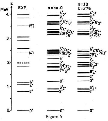
The energy spectrum of Pb<sup>210</sup>. For the range parameter  $\alpha=2$ . calculations with a=b=.0 and a=.10, b=.776 are compared with experimental data. The scarce experimental information does not allow to decide between the two calculated level schemes.
