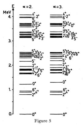
The level scheme of Pb<sup>210</sup> is illustrated. It is shown that the positions of the levels are not sensitive to a variation of the range parameter  $\alpha$  for a = b = .0.
