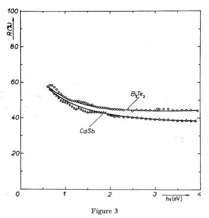
Reflectivity  $R_q$  of liquid  $\operatorname{Bi_2Te_3}$  and liquid CdSb. The full lines were calculated from Drude formulas with the parameters given in the text.
