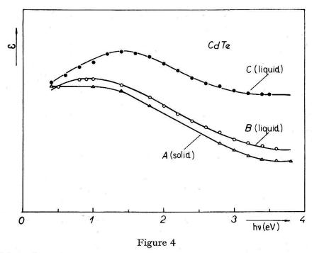
Thermal emissivity  $\varepsilon$  (in arbitrary units) of CdTe. Curve A: solid CdTe at a temperature somewhat lower than the melting point B: liquid CdTe at a temperature somewhat higher than the melting point C: liquid CdTe at a temperature about 150 °C above the melting point.
