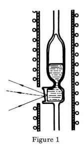
Arrangement for the measurement of the reflectivity of liquids.
