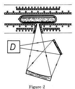
Arrangement for the measurement of thermal emissivity.
