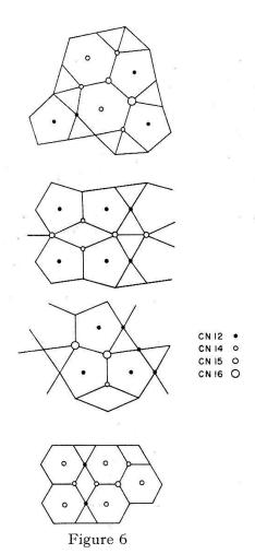
Coordination of atoms of primary and secondary nets for various connections between the net polygons in Frank-Kasper structures.
