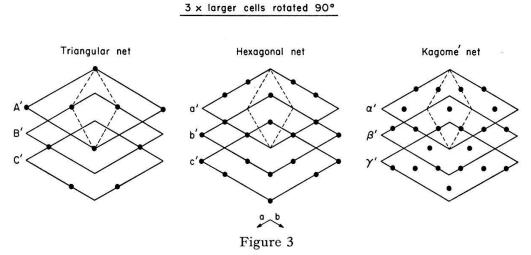
Triangular, hexagonal and kagomé nets of atoms in three stacking positions (A', B', C'; a', b', c';  $\alpha'$ ,  $\beta'$ ,  $\gamma'$  respectively) relative to a basal hexagonal cell which contains respectively 3, 6 and 9 atoms per net.
