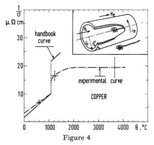
The resistivity of copper as a function of temperature; the insert shows the probe system used  $(r_0 = 0.2 \text{ cm}, l = 3 \text{ cm}).$
