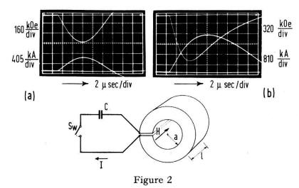
Results of a copper single-turn solenoid coupled to a capacitor bank (Ref. [18]). In oscillogram (a) the field-current relationship is still linear; at higher capacitor bank energies (200 kJ, 15 kV) the field maximum is attained before the current maximum (b).
