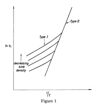
Variation of precipitation time constant  $\tau_1$  with temperatures (schematic). Each type I curve corresponds to one value of sink density.
