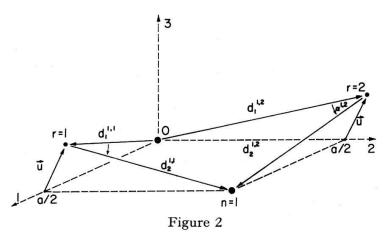
Symbols and coordinate system used in the development of the superexchange coupling constant  $I_{on}$  in terms of the relative sublattice displacement u.
